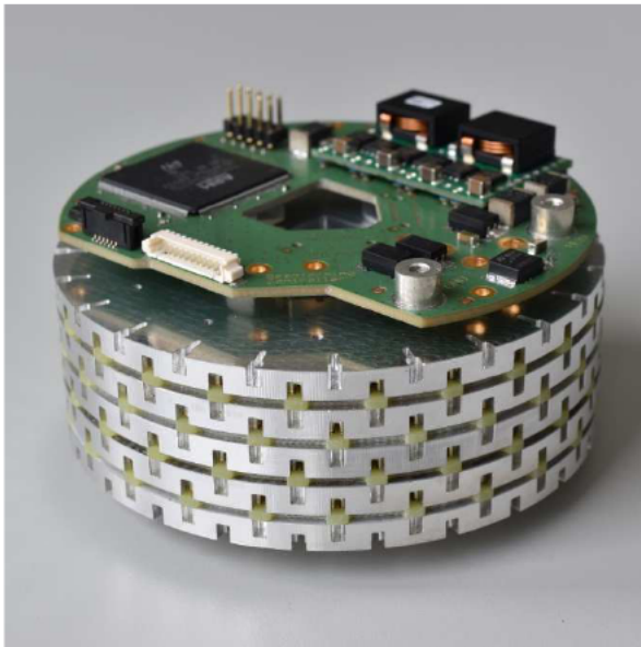
Figure 3: Antenna module for mmWave 5G/6G with the control board on top.
