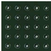
Fig. 2. 5 μm bump, 15 μm pitch Indium bump array
