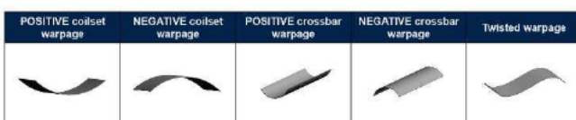
Fig. 3. Strip warpage classification.
