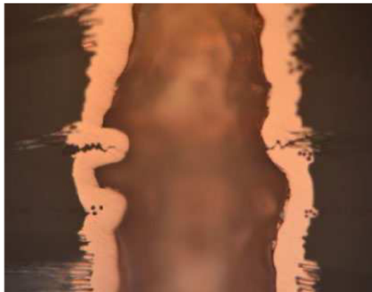
Fig. 7. Metallization damage in the through hole of coupon no. 13.
