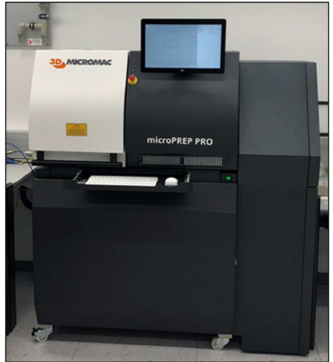
Fig 2.: MicroPrep Pro™, that can be used for efficient laser preparation.
