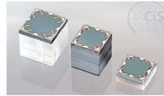
Figure 1 Pressure sensor thickness in correlation to the manufacturing method (from left to right: anodic bonding, silicon direct bonding and SiCer technology)
