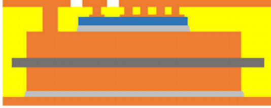
Fig. 6. Schematic of embedded (SiC) prepackage with integrated safety isolation
