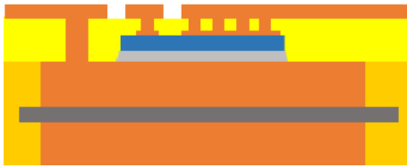
Fig. 2. Schematic of embedded structure with ceramic isolation layer
