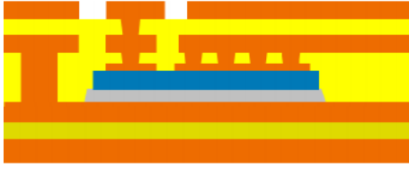
Fig. 1. Schematic of embedded structure with organic isolation layer
