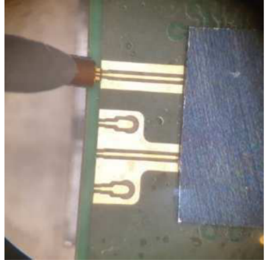
Fig. 10. RF probe landing on package under microscope during measurement
