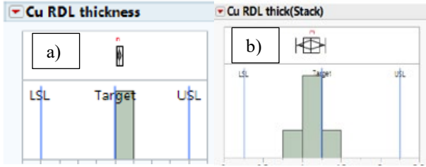
Fig.10: a) RDL thickness after plating, and b) RDL thickness after etching.
