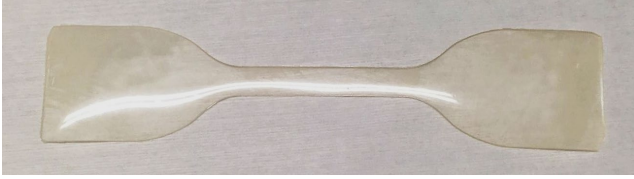
Fig. 4 Test specimen according to DIN EN ISO 527-3 [5] with shape of Type 5 and thickness of 200 \mu\text{m}
