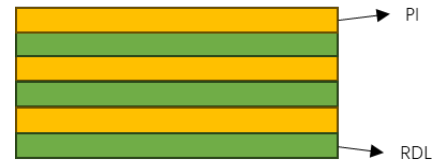
(b) Multi-layer RDL equivalent
