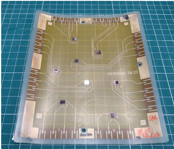
Figure 7: Finished array with 8 embedded sensors
