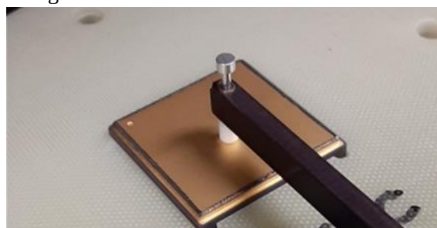
Figure 9. Package and cover in custom fabricated nest for seam sealing.
