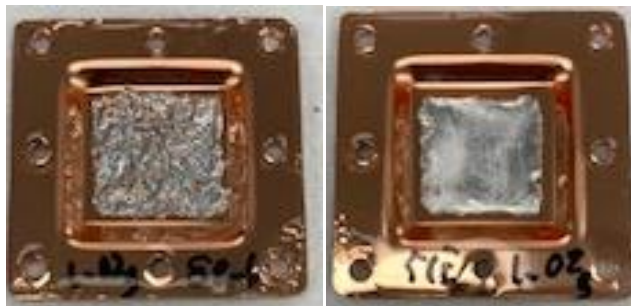
b. After encapsulated with silicone elastomer
