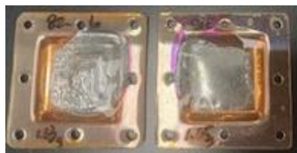
d. HAST with a profile of 264hrs, 110°C/85RH%
