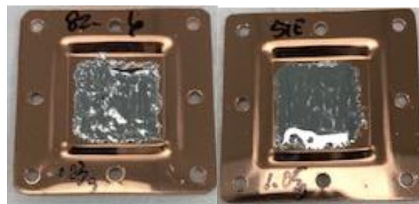
a. Before encapsulated with silicone elastomer
