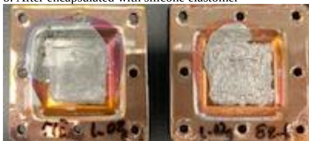
c. HAST with a profile of 264hrs, 110°C/85RH%
