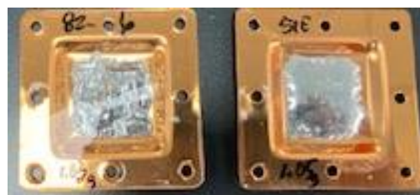
c. Post-treatment at 85°C, 36mmbar/24 hour, N 2 /1week
