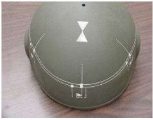
1 st to print conformal antennas
