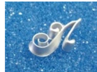
1 st to use a paste to print metal 3D structures
