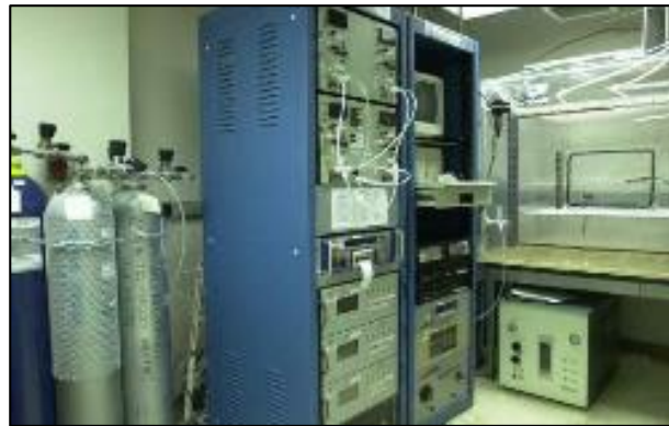
Mixed Flowing Gas Corrosion
