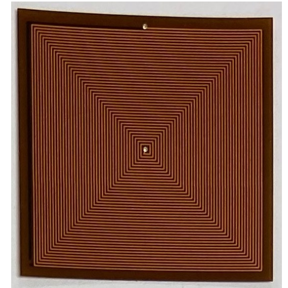
Planar inductor on other side
