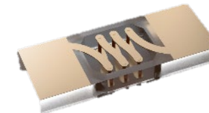
World's best High Q Inductor (SMD) Q=145 @1GHz, 1nH, 0603mm
