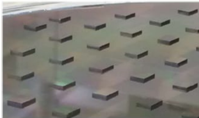
Demonstrator A - 300mm Hybrid Bonding, 5 mm x 7 mm
