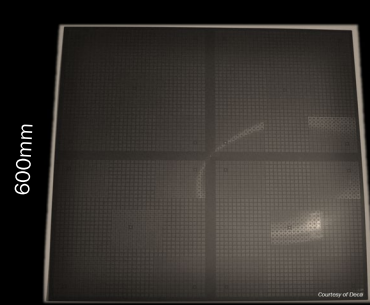
Planarized molded panel (Cu studs exposed)
