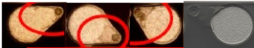
Delamination and discoloration observed after reflow
