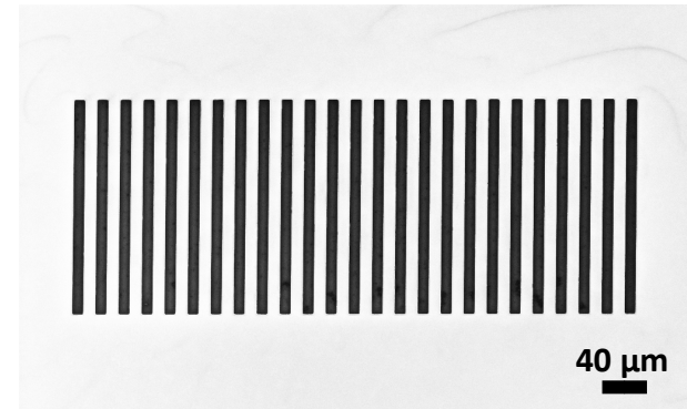
Dielectric channels (10x200 microns and 50 nm thick)
