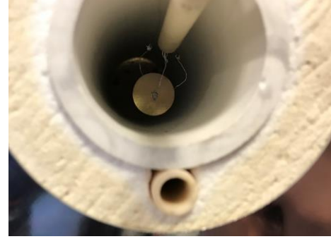
Fig. 5 - PT hanging from ceramic rod in furnace
