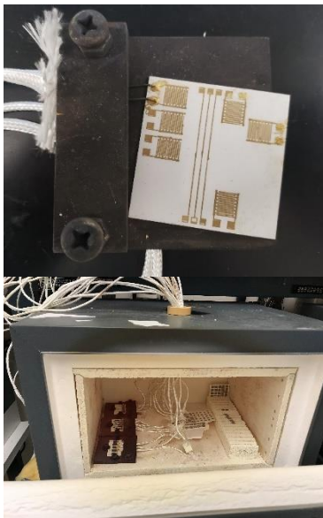
Figure 3 Sample wire attach fixture after 24 hours at 750°C and high temperature storage test furnaces
