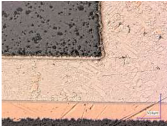
Fig. 3 Solder joint BiSnAg+Cu produced with BSA-01 profile (1000x)
