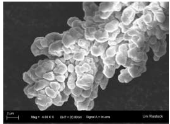
Fig. 2 Agglomeration of copper particles (4000x)
