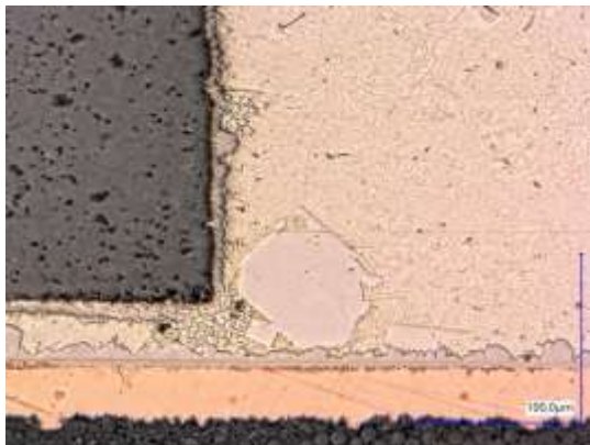
Fig. 10 Solder joint BiSnAg1 produced with BSA-01 profile and thermal aging 168h at 175 °C (1000x)
