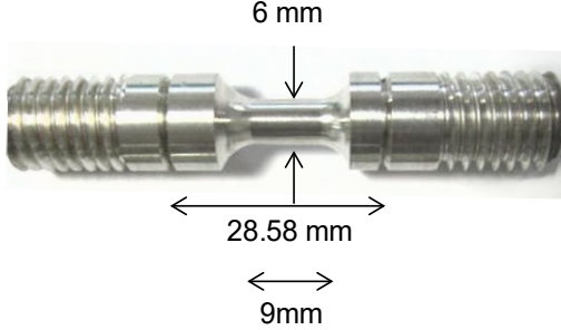
Fig. 2: Specimen for creep test
