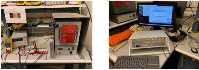
Fig. 1 ASIC setup with 300°C chamber, probe connections to test system (outside chamber), and test equipment
