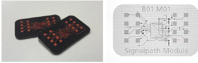
Fig.14: Singulated high temperature embedded modules; photograph (on the left), X-ray image (on the right).
