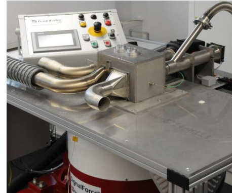
Fig. 28: Test rig for combined vibrational and thermal load
