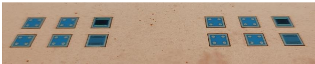
Fig. 15: ceramic platelets integrated in and electrical contacted with the PCB using the sinter lamination technology.
