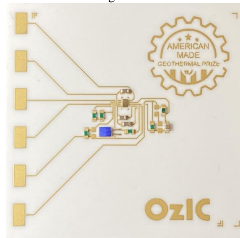
Figure 4: Finished circuit after component attach and wirebonding.
