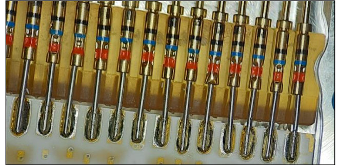
Figure 3: Wires with Pin Contacts Soldered to a Ceramic Wiring Board and Seated in a 3D Printed Isolator Block
