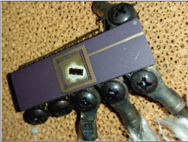
Figure 1: Ad-hoc High-temperature Test Package for SiC CMOS ICs circa 2015 [4]
