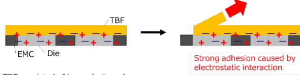
Fig. 1. New polymer system used for the developed TBF.
