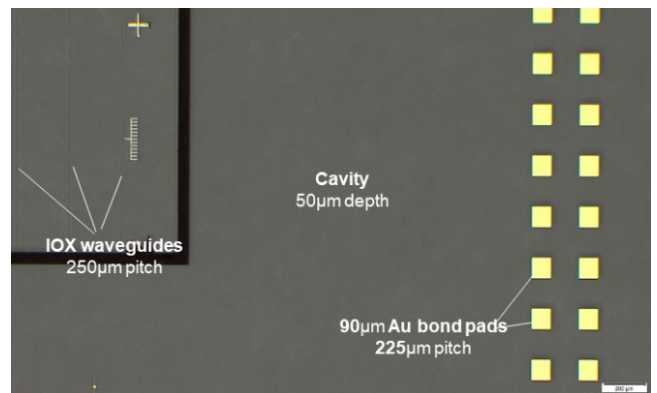
Fig 7. Electrical integration by thin film deposition, spin coating, and contact lithography.
