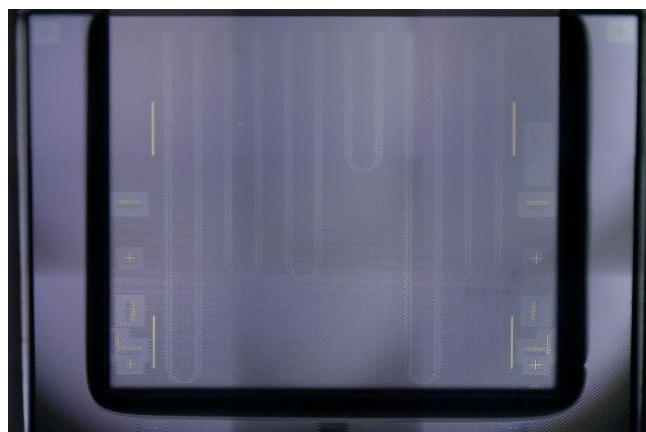
Fig. 10. Top-view optical micrograph of an assembled IOX glass waveguide substrate on a SiN chip. The width of the smaller IOX sample is 3.8 mm.
