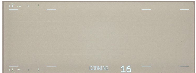
Fig 3. Top view image for 3.8\ \text{mm} \times 10\ \text{mm} \times 0.7\ \text{mm} glass sample with fiducials and an array of 12 waveguides.
