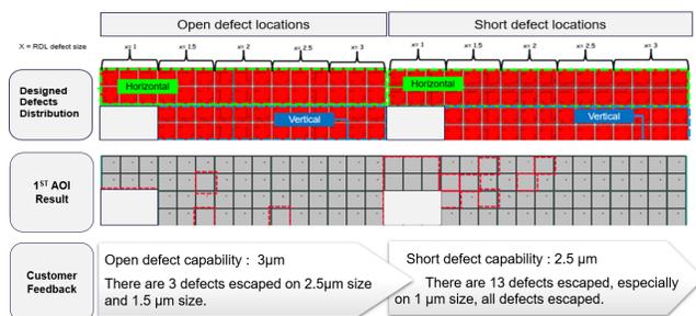
Figure 12. Initial trial inspection result on DOE panel.
