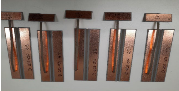
Fig. 6: Peel test layout used for peel strength characterization.
