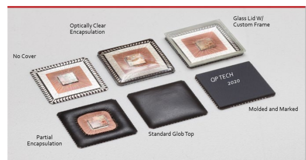
Fig. 3. Encapsulation options for OCPP
