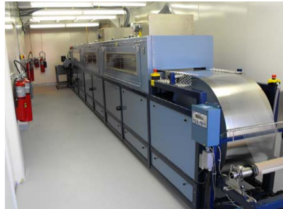
Figure 5: Film fabrication line, oven exit area
