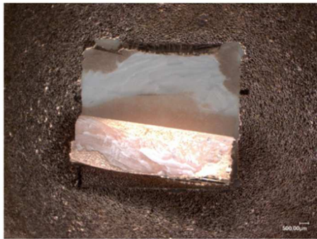
Fig. 8: Optical image of a sheared-off copper foil. The image shows, that the failure occurs at least partly within the ceramic demonstrating the good bonding between copper paste and ceramic as well as between copper paste and copper foil.
