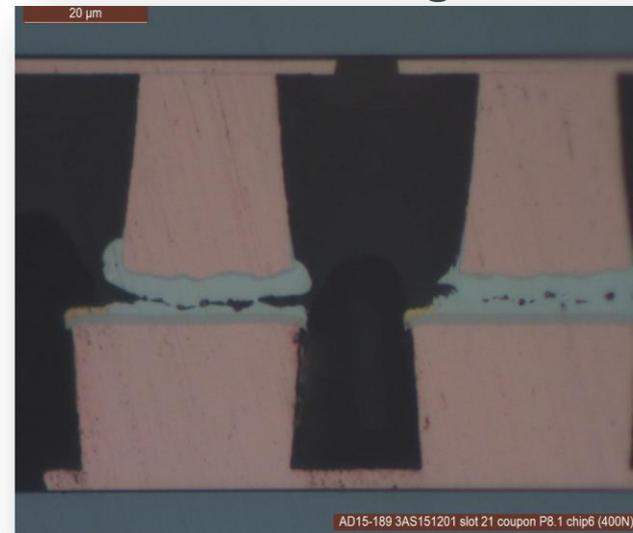
At 36,000 I/O, high viscosity of GEN-1 NCF prevents pillar – pad contact
