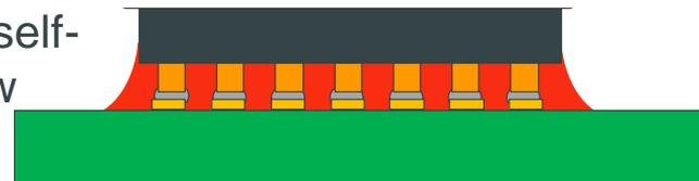
6. Reliability- no filler entrapment in solder joints, correct balance of cured properties (T<sub>g</sub>, modulus, CTE to reduce stress)
