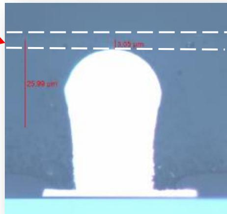
Lamination conditions chosen to minimize NCF layer above solder cap
