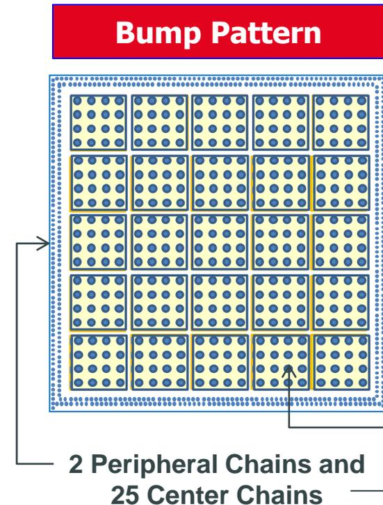
TV-I contains a 25 area arrays and 2 peripheral chains
