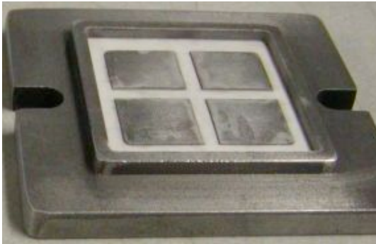
Figure 2. Metal matrix composite module, e.g. AlSiC, with Al-interconnect pads for active and passive components, and terminals. Aluminum on AlN on Al-composite.
