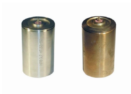
Figure 12: SB-HTA prototype - discharge tests of battery prototypes placed in a diesel fuel fire
