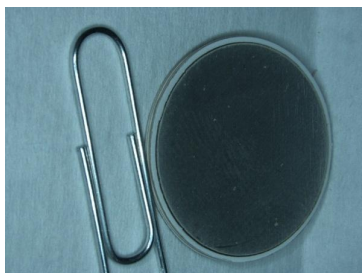
Figure 14: Submillimeter prototype 3.7 V; 25 mAh; Size: Ø 21.5 mm; thickness - 1.1 mm; Safety and fully operability up to 275 °C (527 °F); possibility of recharging at high temperatures.
