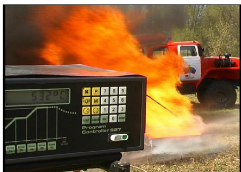
Figure 11: Fire extinguishing; The battery under the fire and hot water vapors
