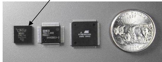
Dice are extracted from the two packages on right and integrated into the package on left.
