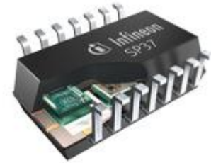
Infineon SP37 Tire pressure sensor for TPMS
