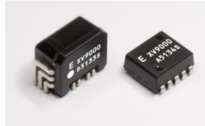
Epson Toyocom XV-9000 series of gyro-sensors for ESC or Rollover
