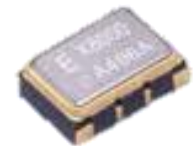
Epson Toyocom XV-8000CV gyroscope for car navigation
