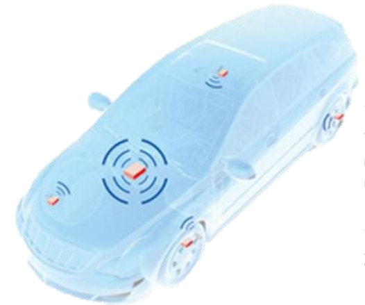
Pressure sensors' position for TPMS, source: Infineon
