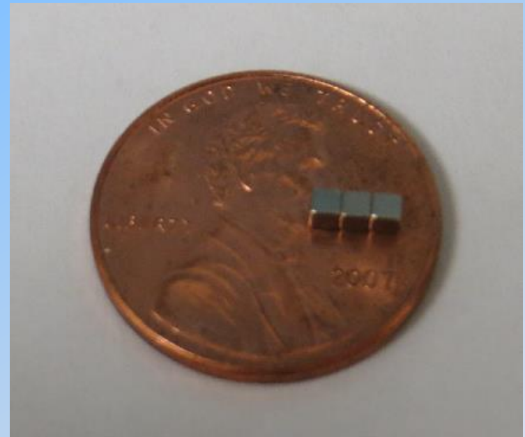
3 miniature Nd-Fe-B magnets on a U.S. penny
