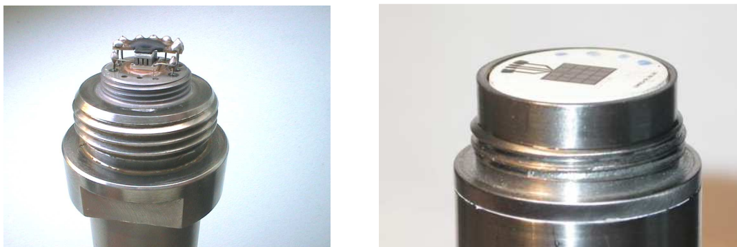
Figure 13: Comparison of CCC* silicon (left) and LTCC (right) dew point probe
