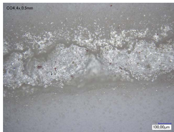
Figure 4: C04 silver lines, nominal line width 0.5 mm, printed on 2 \times 2 in 2 cofired ceramic, four printing cycles
