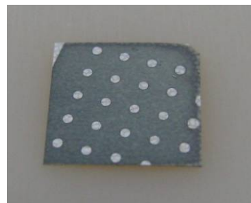
Fig.2 Plate sample of (\text{Ba}_{0.7}\text{Sr}_{0.3})\text{TiO}_3 sintered at 1350^\circ\text{C} for 2 hrs. (Electrodes 0.6\phi , Ag)
