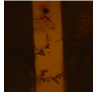
Dendrites caused by electrochemical migration (ECM) of poorly-cleaned flux
