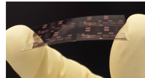
A 125 μm thick glass interposer test die
