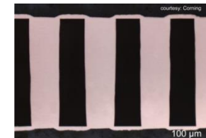
Atotech's double side plating process can fill through holes in panel format with low overburden
