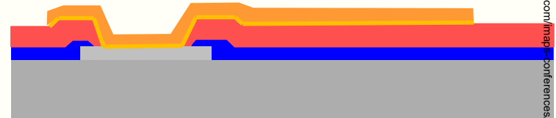
6. Resist Strip & Seed Layer Etch
