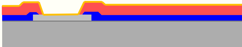
3. Sputtered Seed Layer Deposition
