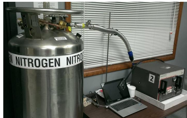
Figure 19: Thermal Cycle Testing Apparatus.
