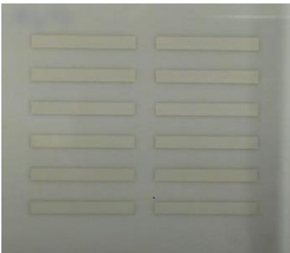
Figure 2: Uniaxial test specimens, (12) 25mm x 3mm x 100 \mu\text{m} thick specimens sintered on \text{Al}_2\text{O}_3 substrate.
